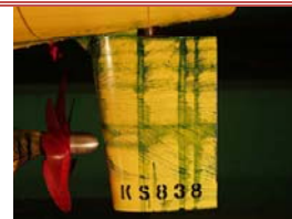
Figure 1.a): Flow paint streaks on the port side of rudder [2]
