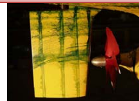
Figure 1.b): Flow paint streaks on the starboard side of rudder [2]
