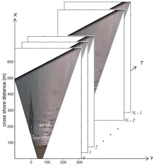
Figure 4: Rectified image time series from snapshot images on 18 August 2006 at 09.00 h around pier area.
