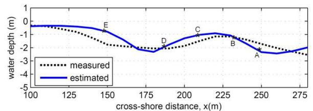
Figure 5: Location of the directional wave spectrum (labeled A, B, C, D, and E) observed along a cross-shore bathymetry profile estimated from video images on August 2006 at Hasaki beach.
