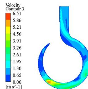
Figure 9: Velocity distribution of volute cross section.
