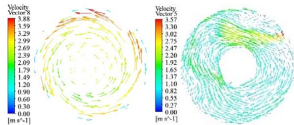
a. inlet pipe b. sliding bearing section
