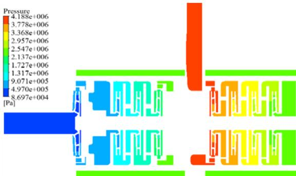
Figure 4: Pressure distribution of the internal flow field.
